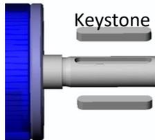
For high alternating loads, torque transmission by positive and frictional locking via a suitable fit or coupling is recommended.
